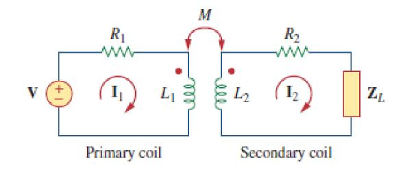
> Apply KVL for loop 1:  $\mathbf{V} = (R_1 + j\omega L_1)\mathbf{I}_1 - j\omega M\mathbf{I}_2$ > Apply KVL for loop 2:  $0 = -i\omega M \mathbf{I}_1 + (R_2 + j\omega L_2 + \mathbf{Z}_L)\mathbf{I}_2$  $I_2 = \frac{JWMI_1}{R_2 + Z_1 + iWL_2}$
