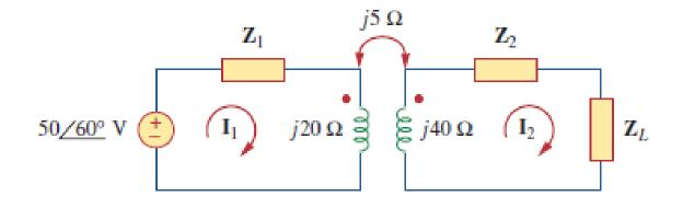
Example6: Determine the T-equivalent circuit of the linear transformer in the following circuit.
