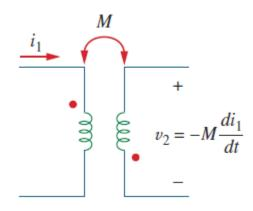
Il enters the dotted terminal of coil 1, V2 is -ve at the dotted terminal of coil 2. so that
