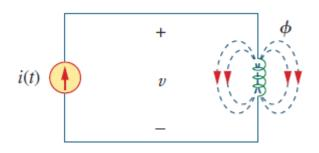
According to Faraday's law, the voltage v induced in the coil is:
