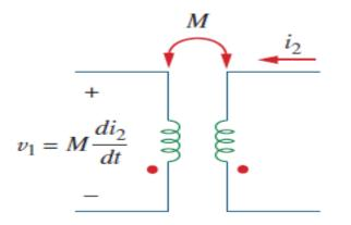
I2 leaves the dotted terminal of coil 2, V1 is -ve at the dotted terminal of coil 2. so that
