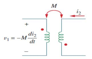
I2 leaves the dotted terminal of coil 2, V1 is +ve at the dotted terminal of coil 1. so that
